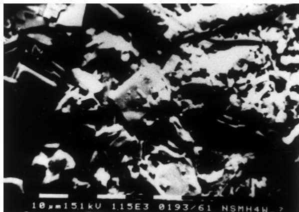
Figure 4 SEM micrograph of polymer pyrrole.
